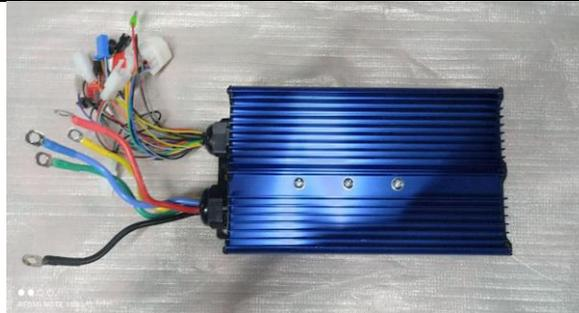
A controller is a device that manages the communication between different parts of a 3W. It is an electronic circuit that controls the speed of the motor in an electric scooter. It receives input from the throttle and precisely controls the flow of current from the battery to the motor.
